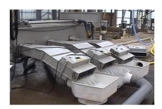
The fish counter inlet is placed to the fish grader outlet
